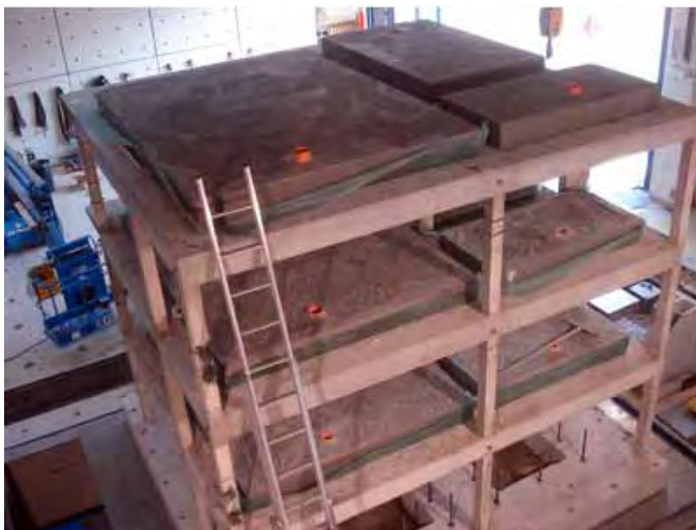
Figure 2–7: Additional mass for the simulation of storey superimposed dead and live loads
