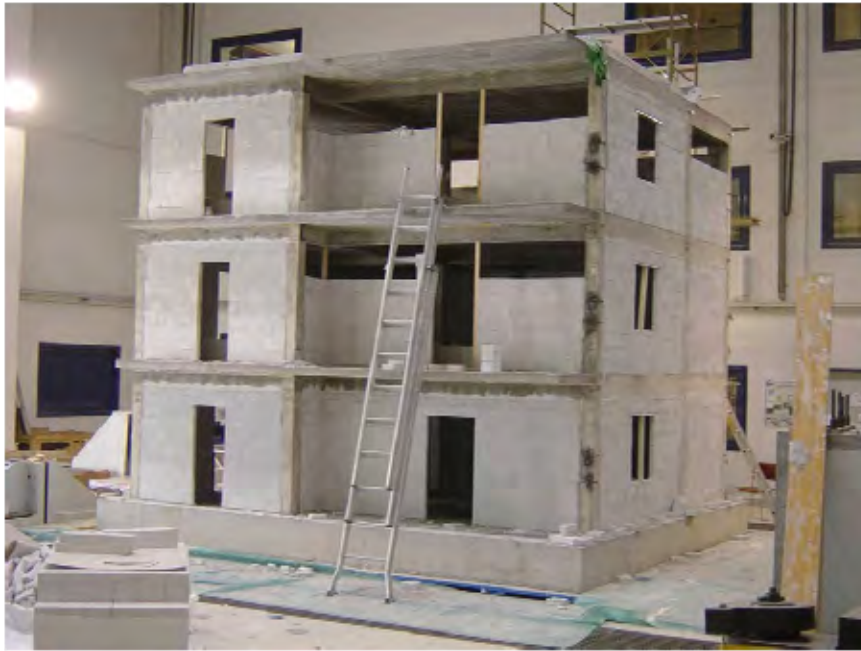
Figure 6–7 Construction of the infill walls
