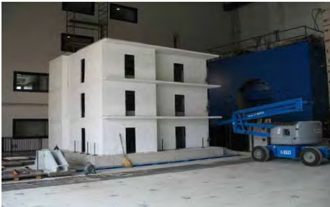
Figure 2–9: The building of the seismic experiment NEARB on the shake table
