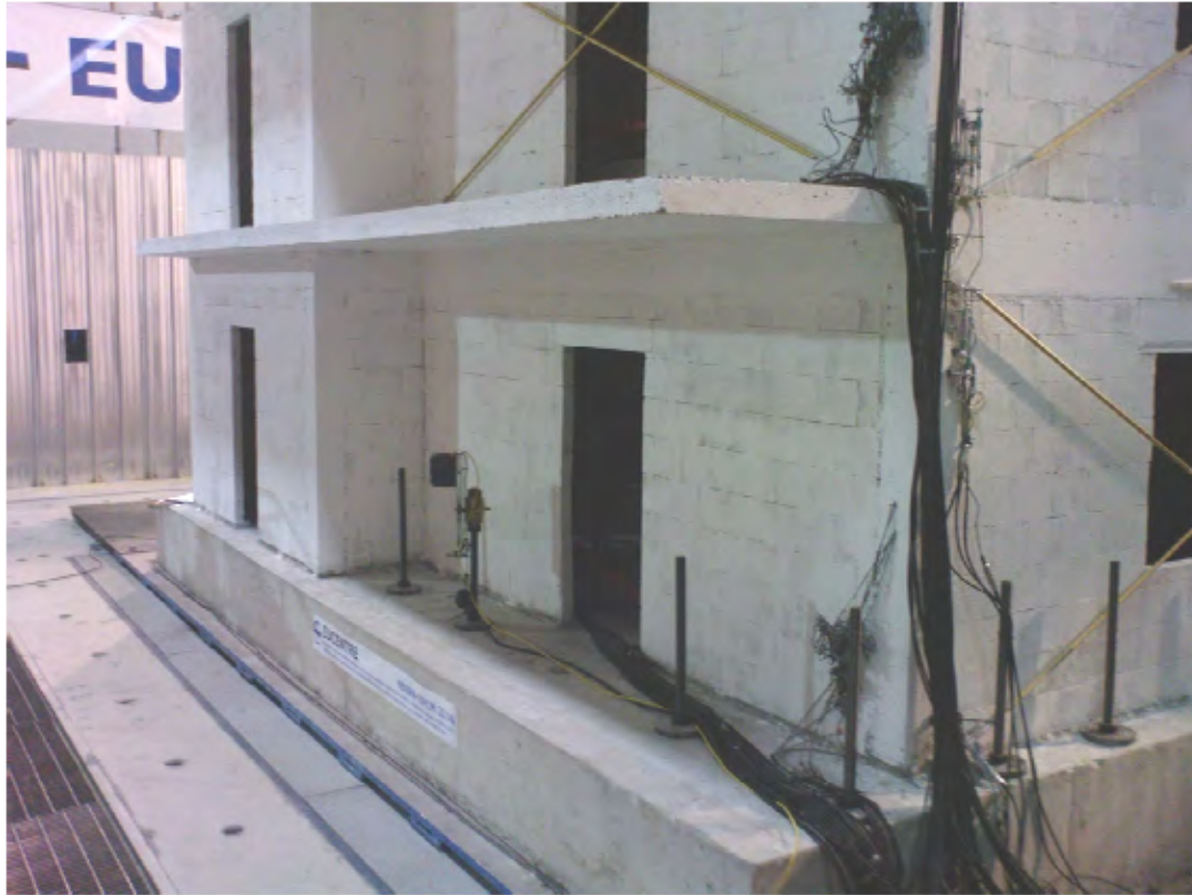
Figure 5-9: Displacement gauges of column C6
