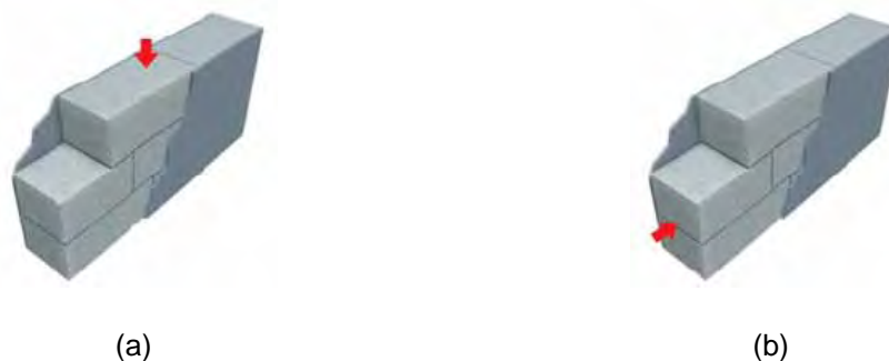
Figure 2-4: compressive strength (a) vertical f_m = 2.2 MPa (b) horizontal f_h = 1.8 MPa
